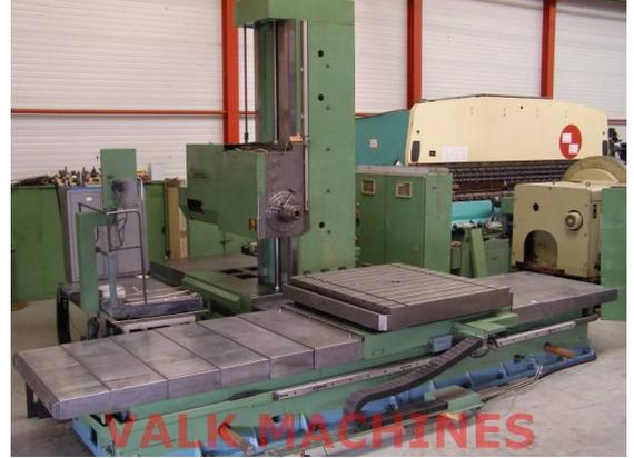
Spindel Durchmesser: 130 mm
